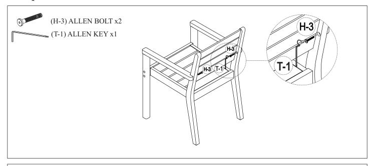
Using Allen Bolts (H-3), and Allen Key (T-1), secure Left Frame Leg and Right Frame Leg (C1 & C2) to Backrest (A) Fully tighten, but do not over tighten.
